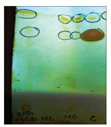
**Figure 3:** Thin Layer Chromatography (TLC) showing equal distance run by MBEH and Mobile cover component.
